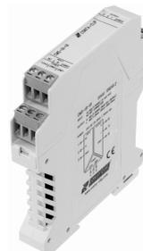
The CMS-UI-UI is a multi-functional 3-way isolated signal converter. This module is used for electrical isolation and conversion of analog signals. The 3-way isolation enables the module to be used locally as well as in the vicinity of the controlling system.
